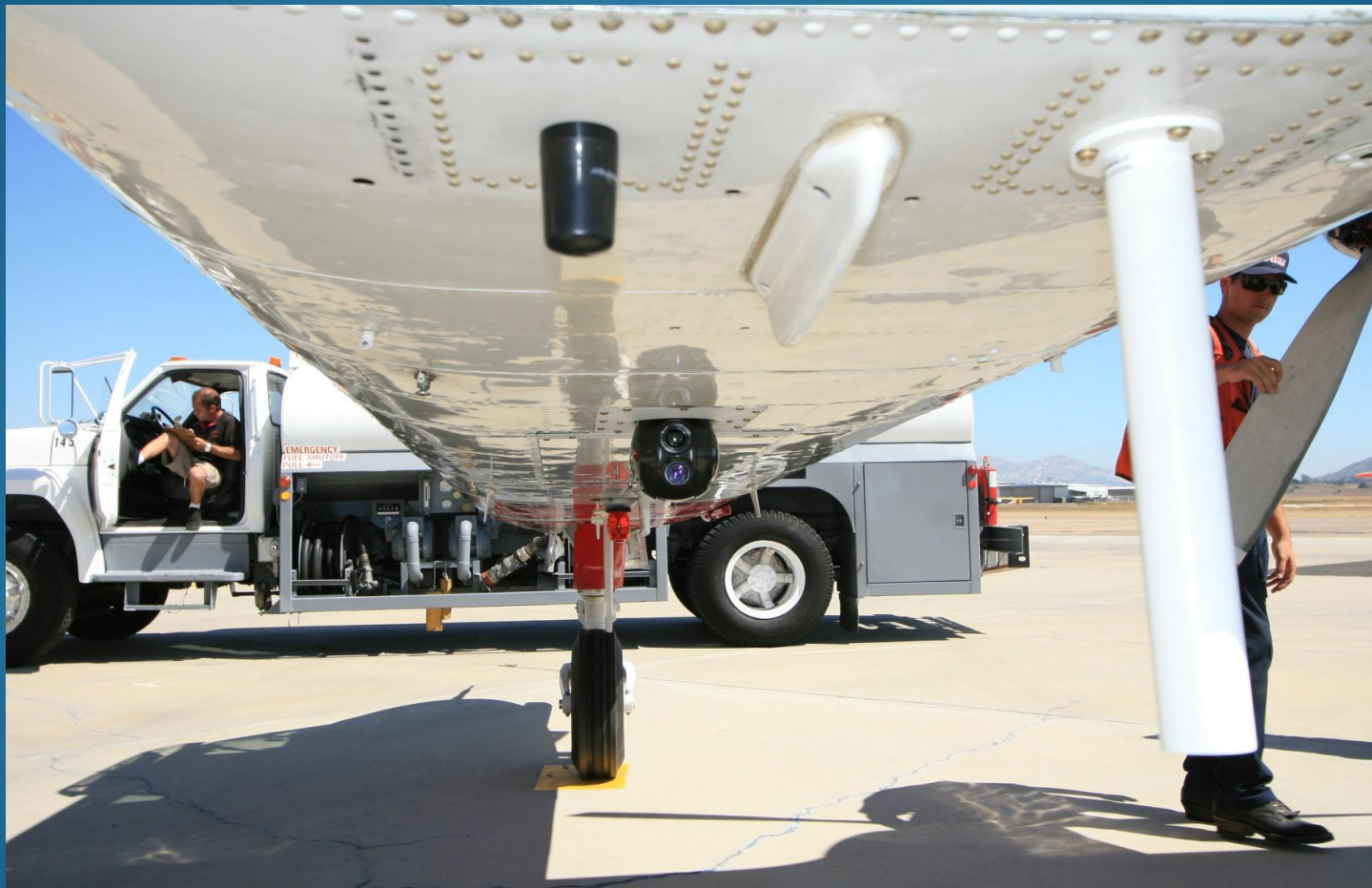
IR/ Video Camera mounted on AA-330
