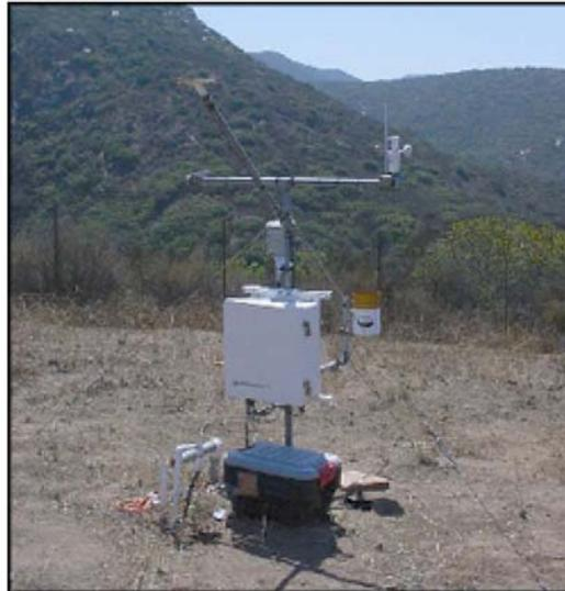
*Figure 3.* Located near the reserve's north station, this weather station collects data related to wind speed and direction, air temperature and relative humidity, solar radiation, precipitation and atmospheric pressure.
