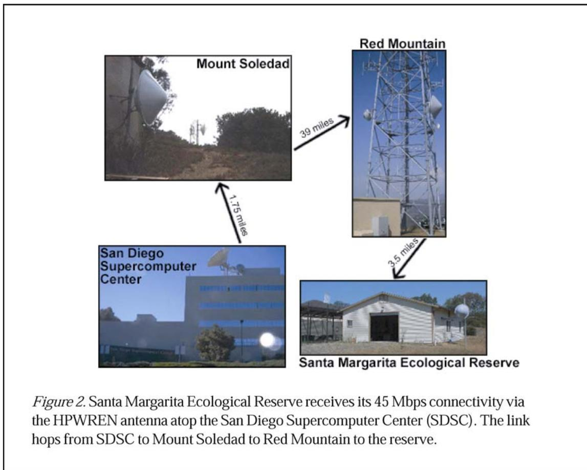
*Figure 2.* Santa Margarita Ecological Reserve receives its 45 Mbps connectivity via the HPWREN antenna atop the San Diego Supercomputer Center (SDSC). The link hops from SDSC to Mount Soledad to Red Mountain to the reserve.
