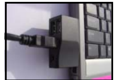
The PCMCIA card should be inserted properly into laptop slot, as shown here.
