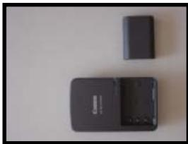
The *camera battery charger* is located in the backpack. After each LIVE session, use the battery charger to charge both of the camera batteries. Once the battery is charged, the orange light on the charger will turn to green. Place one of the charged batteries in the camera and the backup battery and charger back in the backpack.
