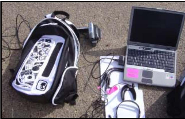
As shown in this image, the camera cable connects the DV camera to laptop's firewire slot in the PCMCIA card. The dual audio adapters are connected between the laptop and the audio components.
